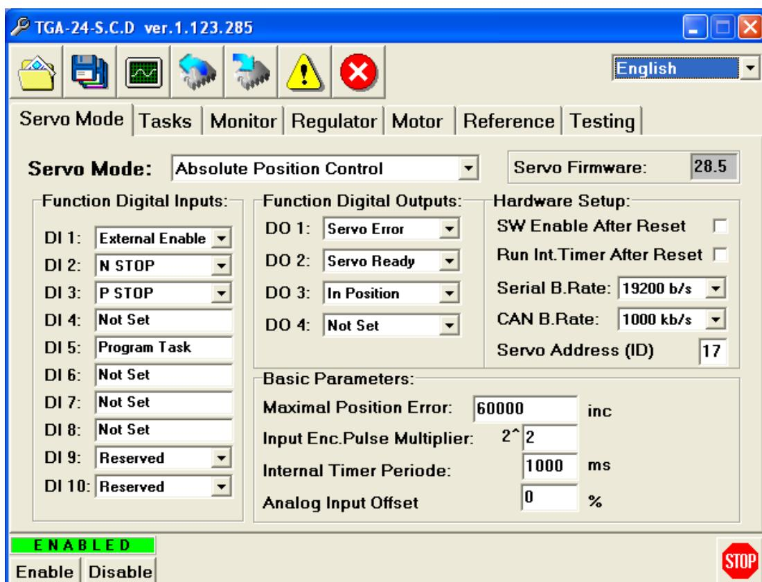
It is possible to program 10 functions to the servo controller. The functions can be started by rising or falling edge of a digital input, internal timer, or signal In position or Speed=0.
