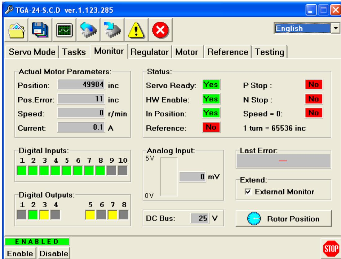
Menu Monitor allows monitoring status and parameters of a servo-controller (inputs, outputs, input voltage, faults) and a servomotor (position, position error, speed, current, faults). To see the value in other modes it is possible to enable External Monitor and External Monitor window is opened.
